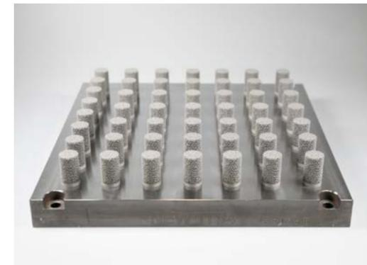
Figure 7: The build job contains cylindrical lattice specimen on the entire build plate.
